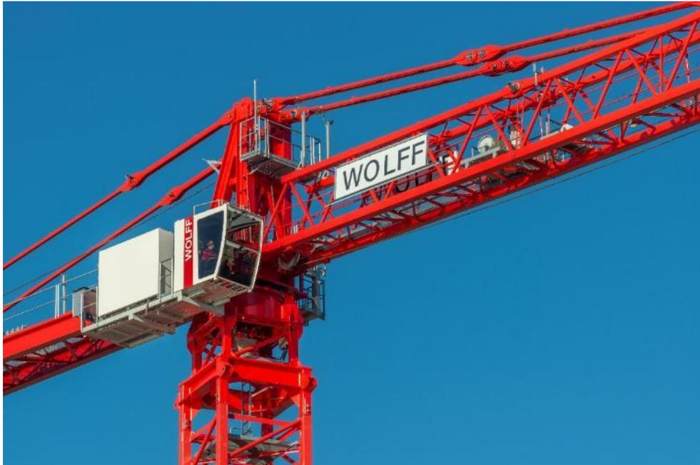
The compact tower top allows several cranes to stand close together on a construction site and slew over each other.
