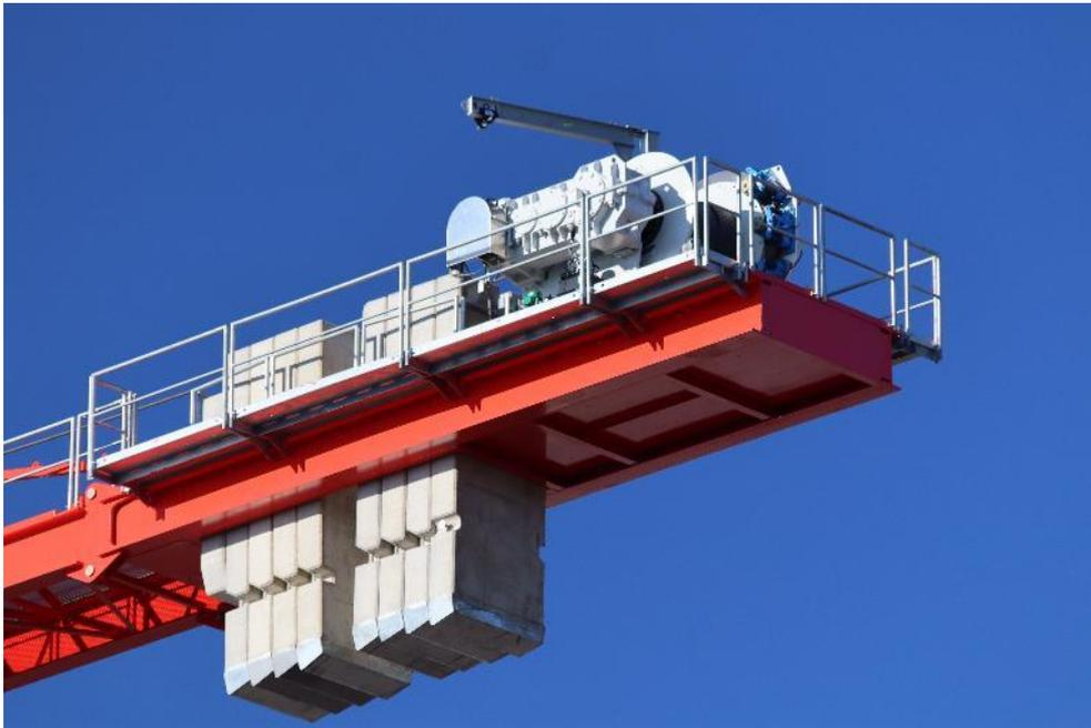
To the right of the counterweight blocks is the proven and most powerful HW 40132 FU 132 kW hoisting winch, with which operating speeds of up to 95 m/min are possible. At the top is an auxiliary crane for service work.
