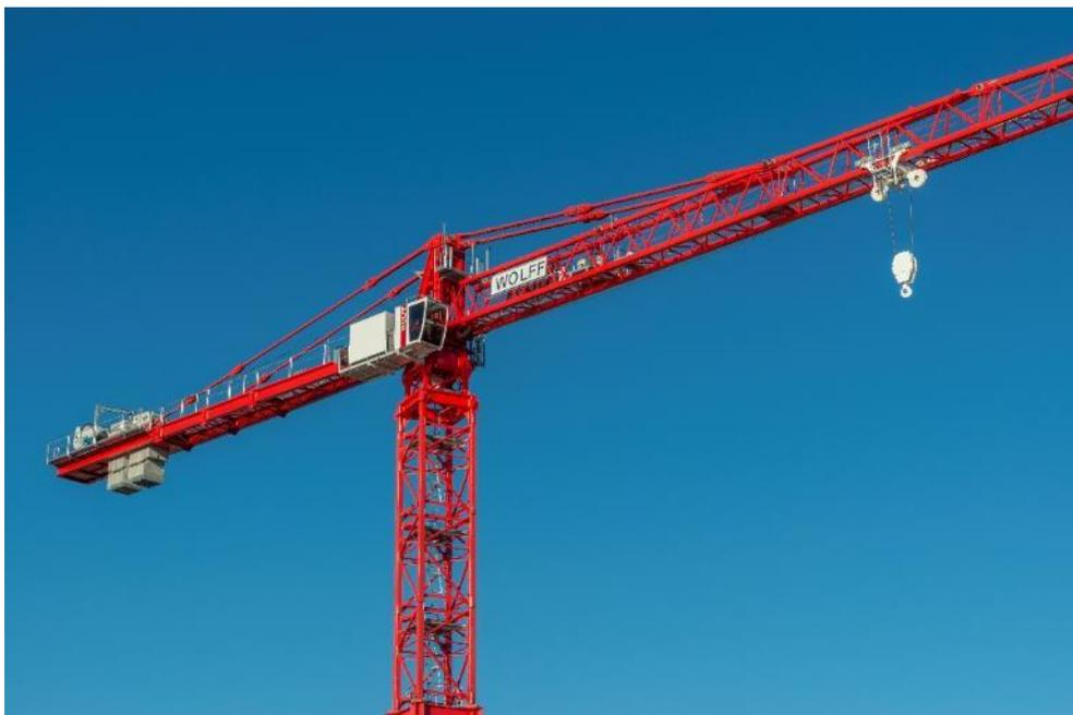
With the low-top design, WOLFFKRAN engineers get the maximum lifting capacity out of the crane. The WOLFF 8076 Compact lifts up to 40 tons.
