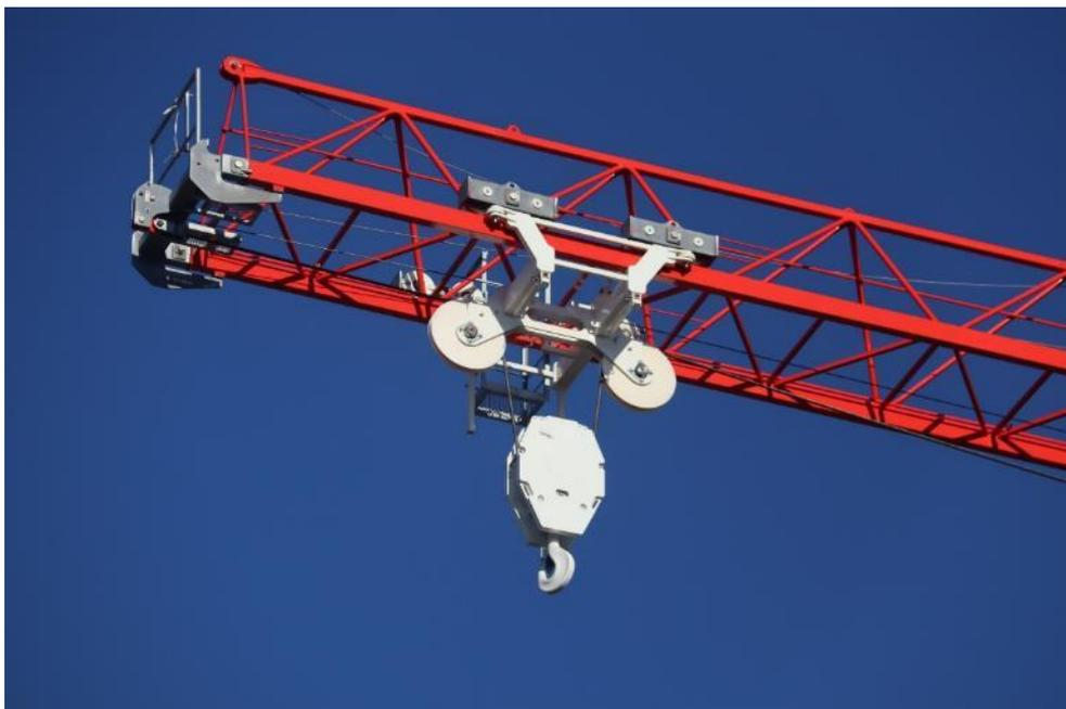
The WOLFF 8076 Compact is launched on the market as a pure 2-fall crane. Despite this, it still lifts 8.4 tons at the top with an 80-meter jib.
