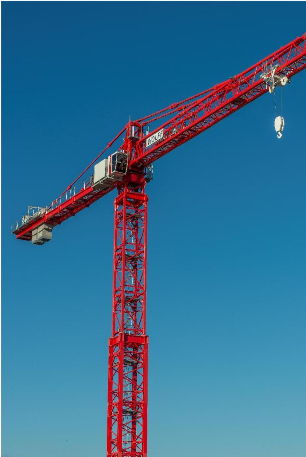
Combined with the next largest WOLFF tower element TV 33, free-standing tower heights of up to 100 meters are possible.
