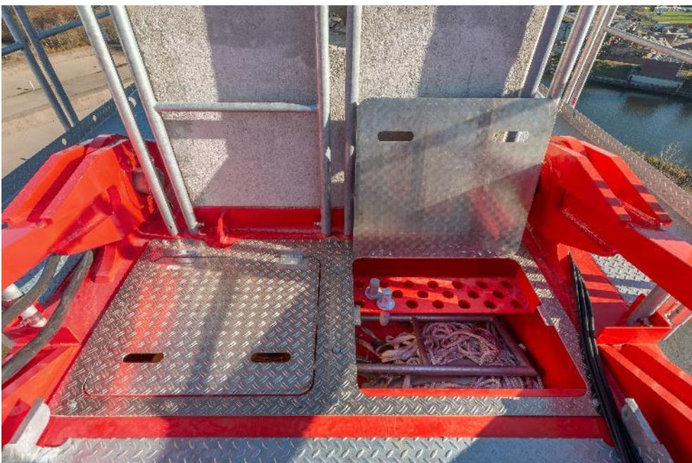
Stowage space with depot for stub shafts for the counterweight blocks.
