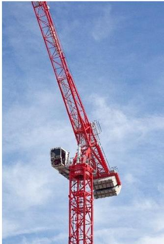
The WOLFF 166 B US is fitted with a compact hydraulic luffing mechanism.
