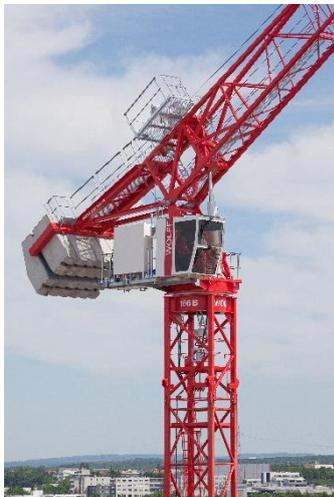
The WOLFF 166 B US comes with the latest WOLFF CAB crane cabin.
