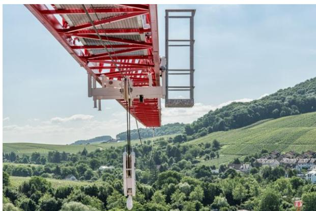
WOLFF engineers redesigned the trolley by replacing the rollers with wheel flanges used to date by rollers without wheel flanges and a new guide roller on the jib, thus optimizing the run of the trolley.
