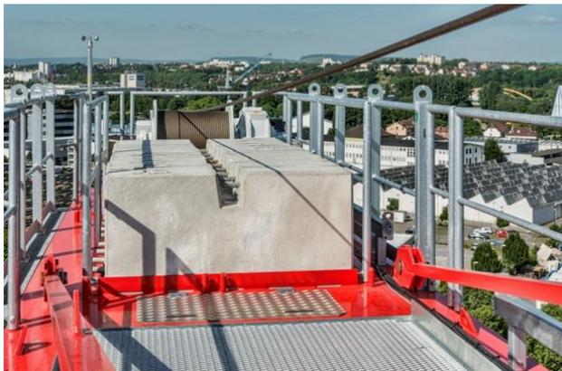
The counter jib has been fitted with new railings that are suitable for attaching safety harnesses thus improving the safety for technicians working on the counter jib.
