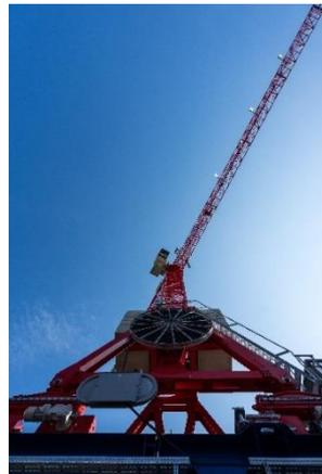
Clever, thoroughly considered solutions were necessary due to tight space constraints at hand. The cable drum is located on the exterior of the gantry.
