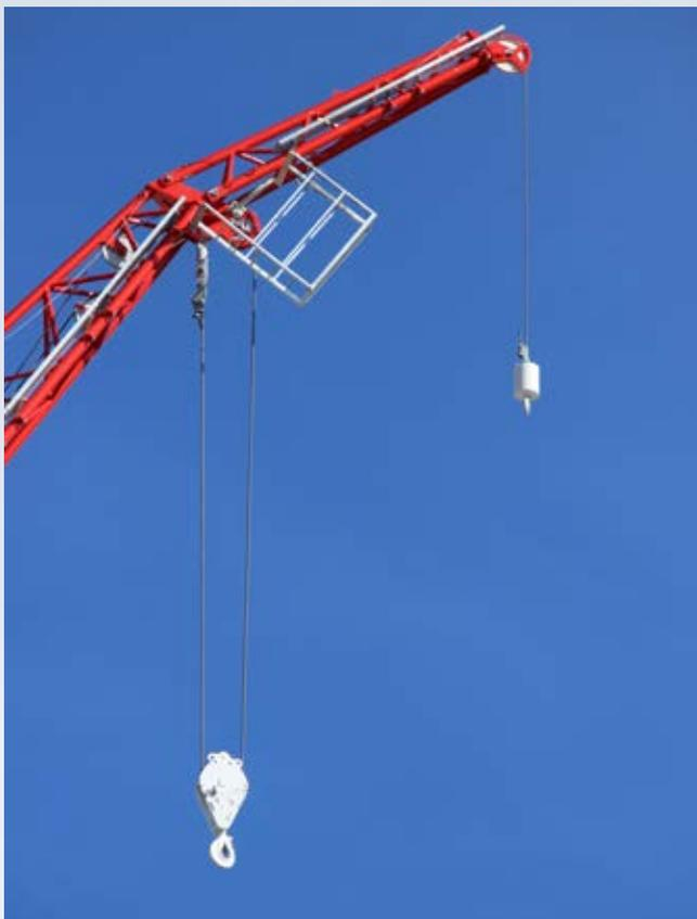
As a special application all our latest generation WOLFFKRAN cranes have the option of using an additional fly jib. Our technologically advanced solution provides an additional hook with an 8t capacity at a range of 5m beyond the main hook; ideal for lifting unconventionally large and long loads, offering precise turning and positioning capabilities. Offering you the perfect view and ultimate control for the complex demands of wind turbine storage yards.
