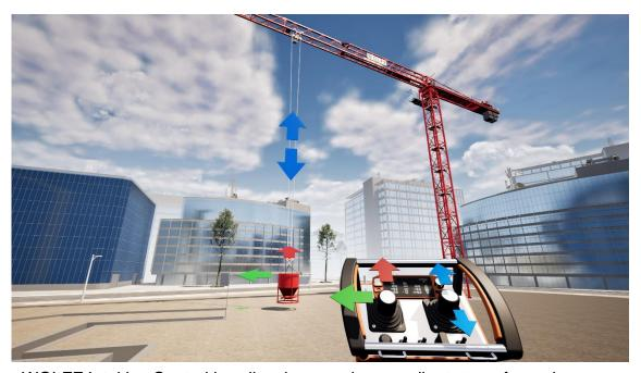
WOLFF Intuitive Control handles the complex coordinate transformation automatically and allows the operator to steer the load directly in the desired direction. For greater convenience and safety on the construction site.
