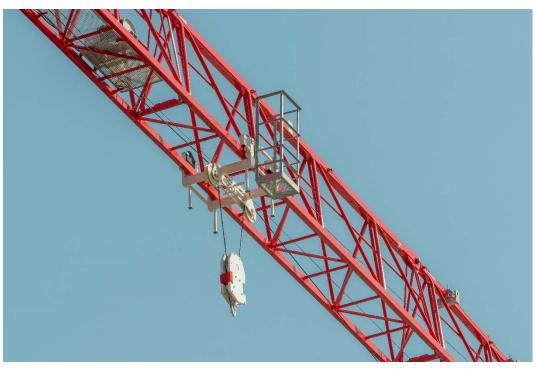
Thanks to this re-design of the jib lower chord, assembling the WOLFF 6523 Clear is made easier and the trolley runs more smoothly along the jib.
