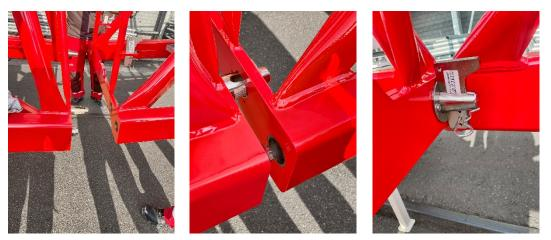
Instead using a bolt connection, the jib sections are mounted on the front with a mandrel and wedge connection.
