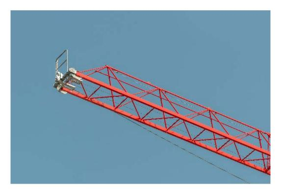
The rope swivel traverse at the tip (above) has a mandrel and wedge connection thanks to its new lower chord jib design, making it easier to assemble. Its railings and walkway grids are galvanized, making them exceptionally robust and long-lasting.
