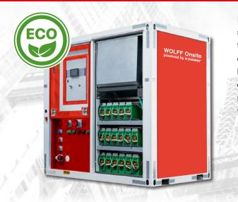
Introducing the WOLFF Hybrid Power Unit, an innovative solution that combines a battery and a diesel hybrid generator to reduce fuel consumption by up to 90%. The energy management system optimises power delivery dynamically, with the battery taking on peak loads and the generator recharging it efficiently. This hybrid generator is designed to adapt to weak grid connections and consume minimal energy, making it an eco-friendly and cost effective energy management solution for construction sites.
